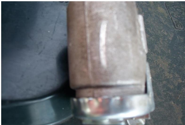
dave and I will come and have a look he said. After investigation Nigel hit on the problem. What was happening was where I had fitted a replacement (pattern) wheel cylinder on the nearside rear wheel the wheel bolts were catching on the outside of the cylinder(see picture). This can only happen on the Series
