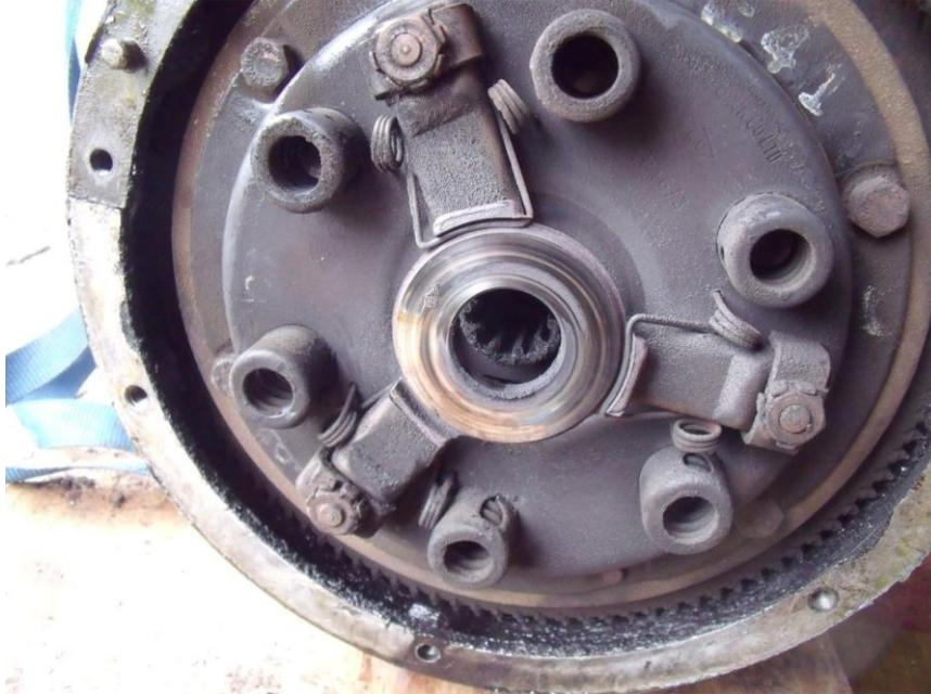
Original clutch before removal. Note the broken release lever spring.
